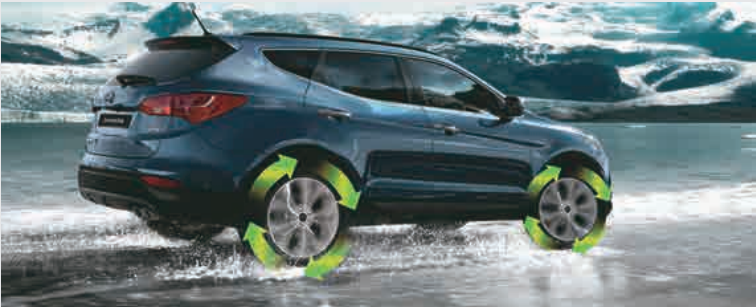
TCS (Traction Control System): Maintains control during wheel spin especially during slippery road conditions.
