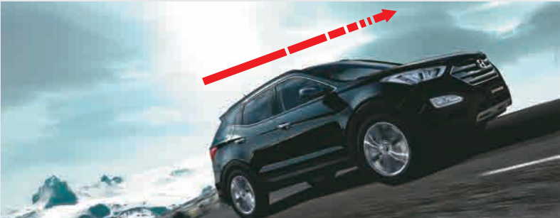
HAC (Hillstart Assist Control): The HAC helps in detecting an incline and brakes are automatically engaged to prevent dangerous roll-back.
